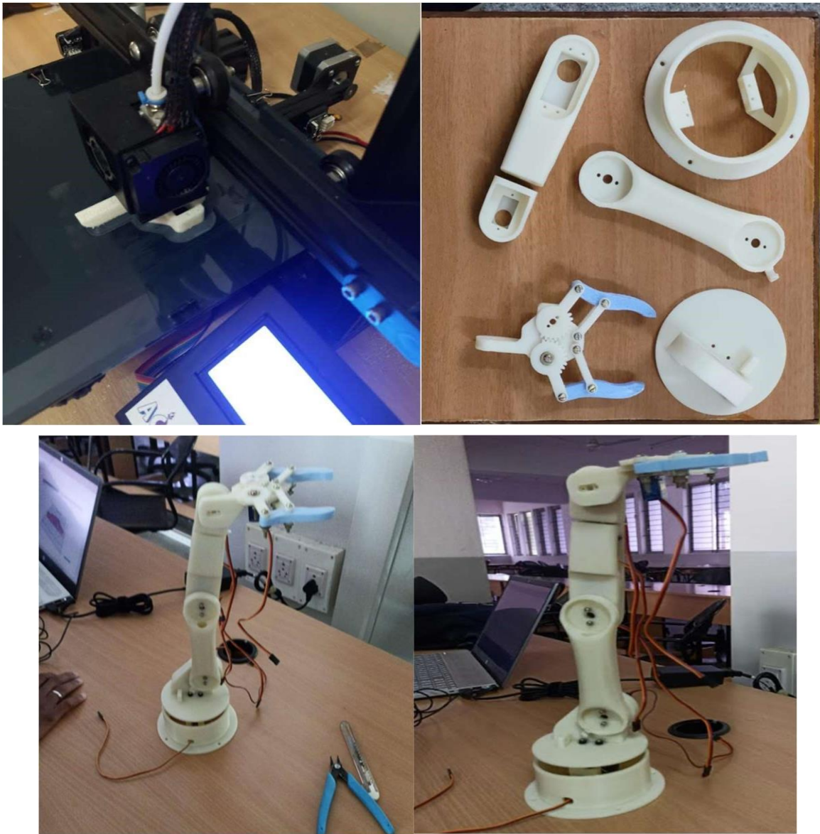
Figure: Final Testing and Inspection of 3D printed Robotic Arm
